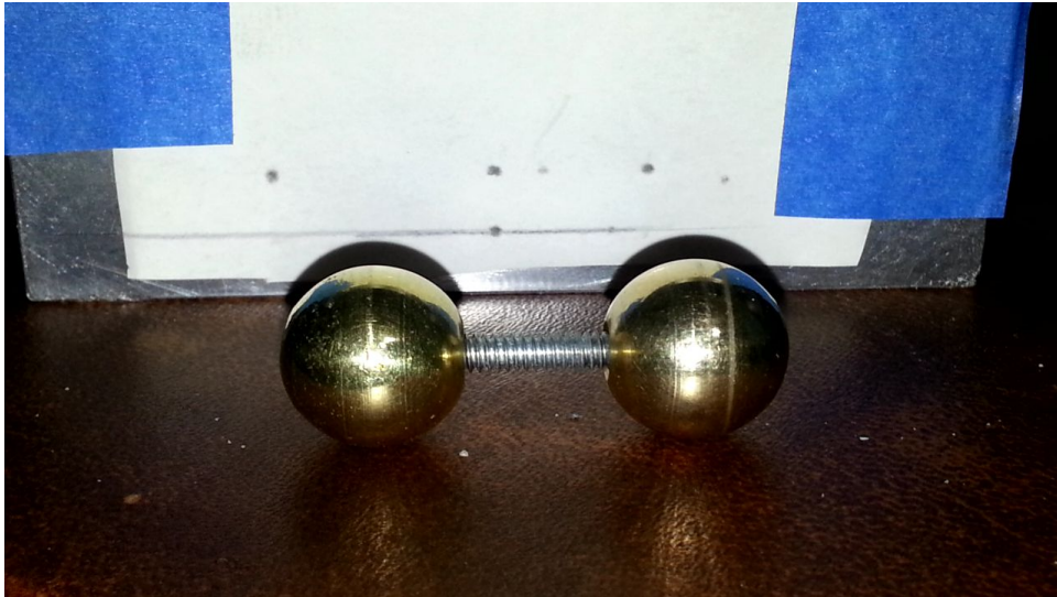
FIG. 1. Custom made Hurricane Balls and thermal paper affixed to vertical metal plate. Commercially available Hurricane Balls are welded together rather than being connected by a shaft. The line across the bottom is a reference line created one ball radius off the surface by dragging the balls across the plate. The strike marks come from slowly moving the plates up to the whirling balls until the upper ball strikes the paper.
